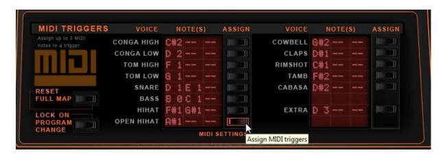
While assigned by default to GM MIDI map, the VPROM triggers can be assigned to any MIDI notes, precisely 3 notes slots are available per drum. However you cannot assign the same note to trigger multiple drum at the same time. It is multiple notes (3 notes max) per Drum and not multiple drums per note if that make sense .
